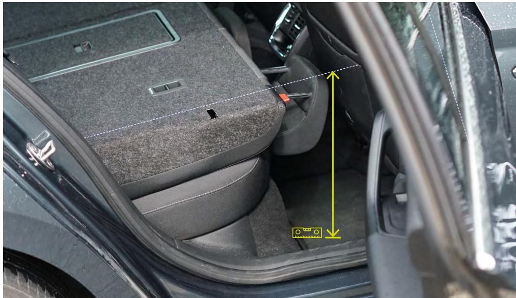
EN Height difference between the folded seats and the floor behind the driver seat (to know needed height of the support legs if placed on the ground)
