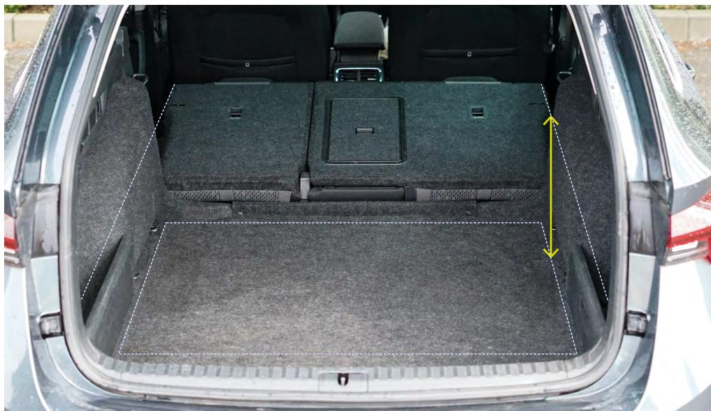
EN Height difference between the boot floor and the highest point of the folded seats
